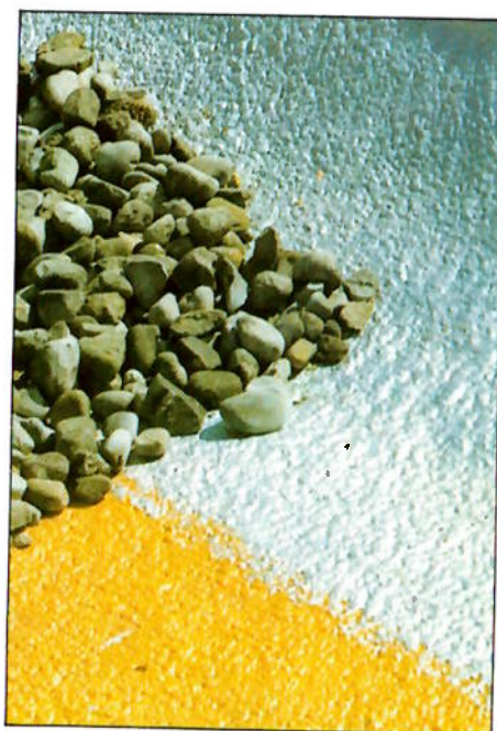
The insulating layer can be covered with a gravel filling (grain size 16/32 mm), or a protective coating based on Desmodur E 22
