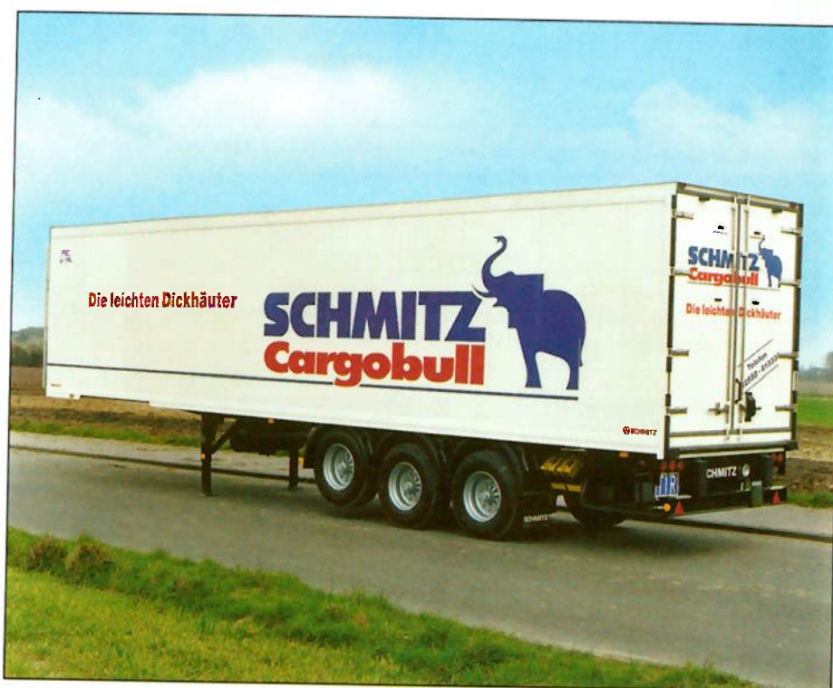
A refrigerated trailer insulated with polyurethane foam and used for the transportation of perishables
